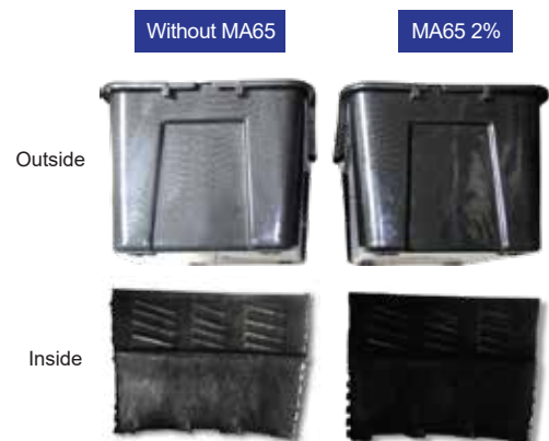
Fig 3 : Comparing extrusion sheet with and without Elastotech ® MA65
